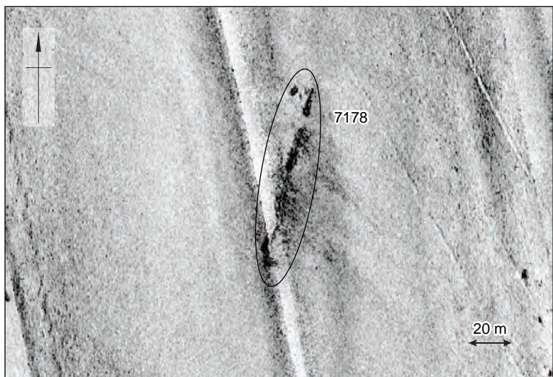
Sidescan mosaic image of seabed disturbance 7178 , measuring 86.5 x 12.5 m
